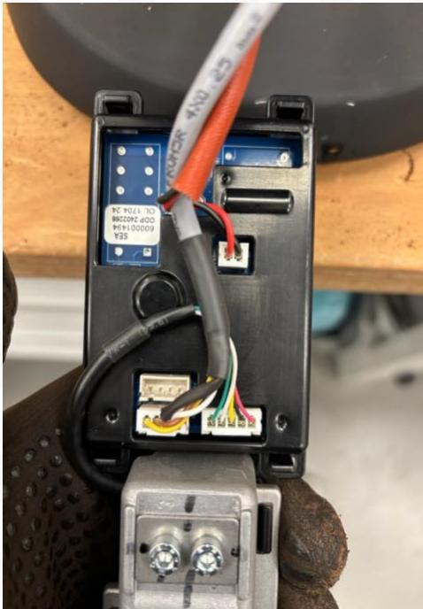
Remove the connections to free up the scale assembly//
