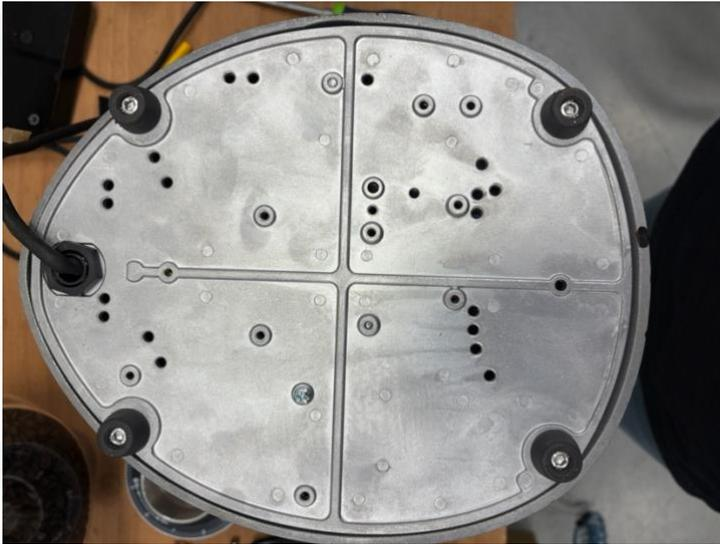
Remove the Hex head screw in order to remove the bottom cover//
